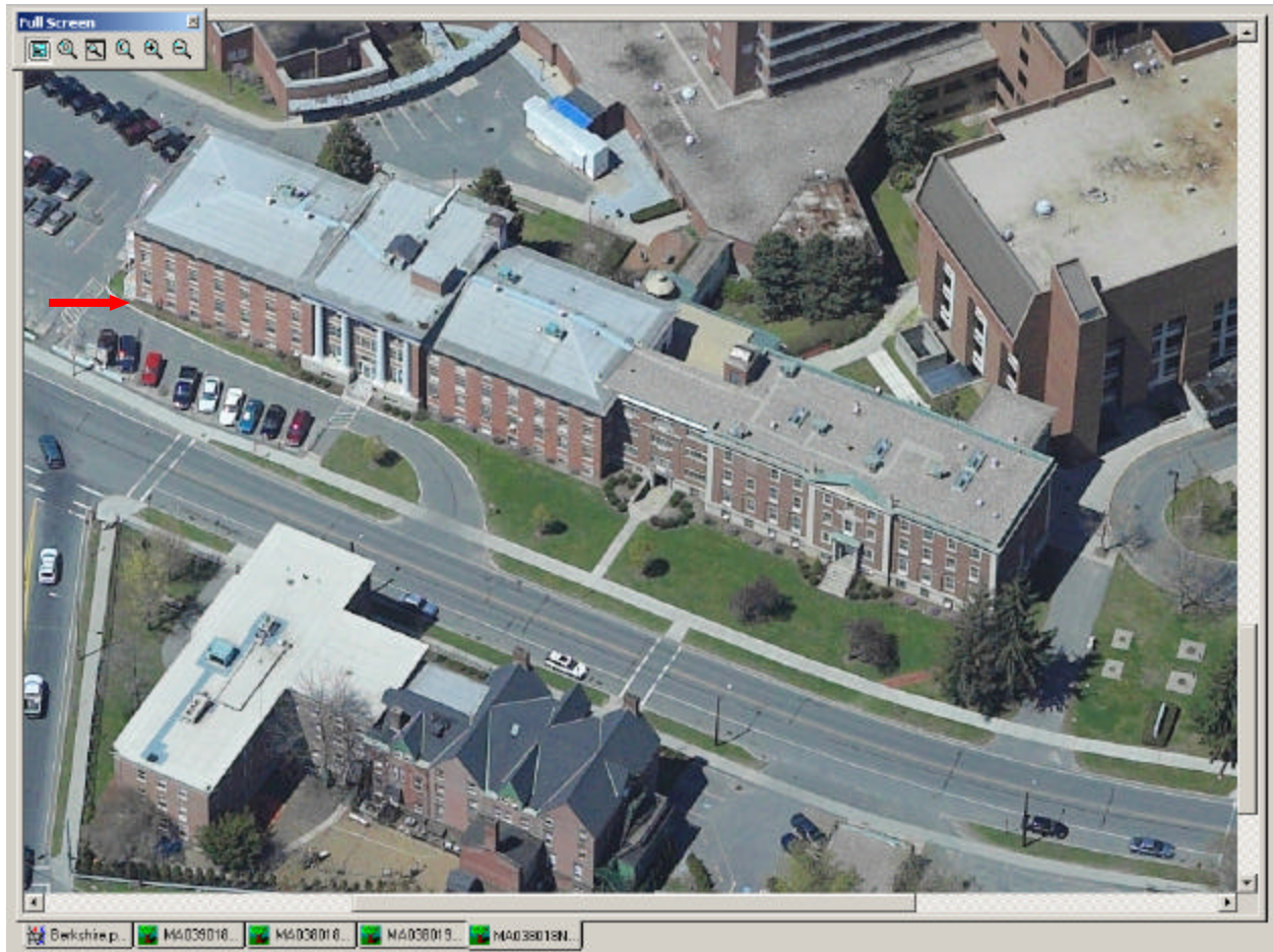
Figure 2: shows the Pictometry interface displaying a color digital oblique-image of a community viewed from the East. This image is shown at the Neighborhood Oblique Scale. The red arrow in the view is pointing to a building that will be the target feature.
