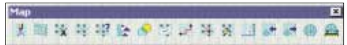
Map Toolbar (from left): Drawing Cleanup • Boundary Break • Boundary Trim • Create Topology • Query Topology • Thematic Mapping • Overlay Topology • Buffer Topology • Shortest Path Trace • Flood Trace • Edit Topology • Plot Map Set • Import Map File • Export Map File • Assign Coordinate System • Geodetic distance
